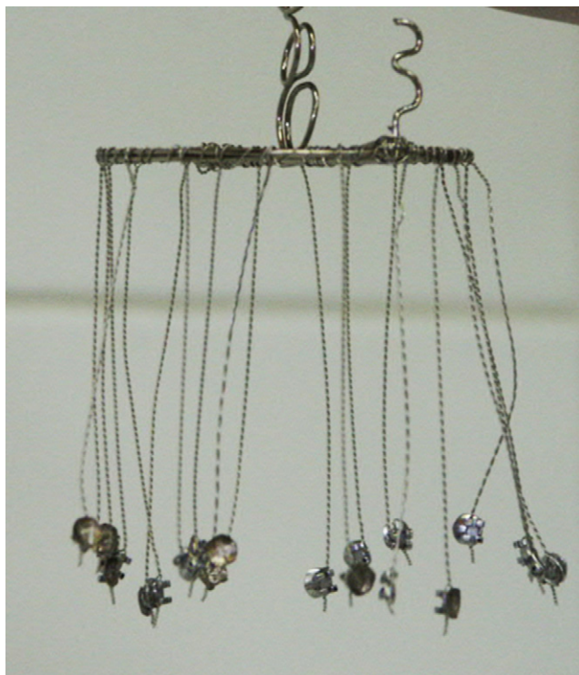
Fig. 2: Brackets of Group 3 attached by .010" metallic ligatures to a .036" round base, making it a single entity.
