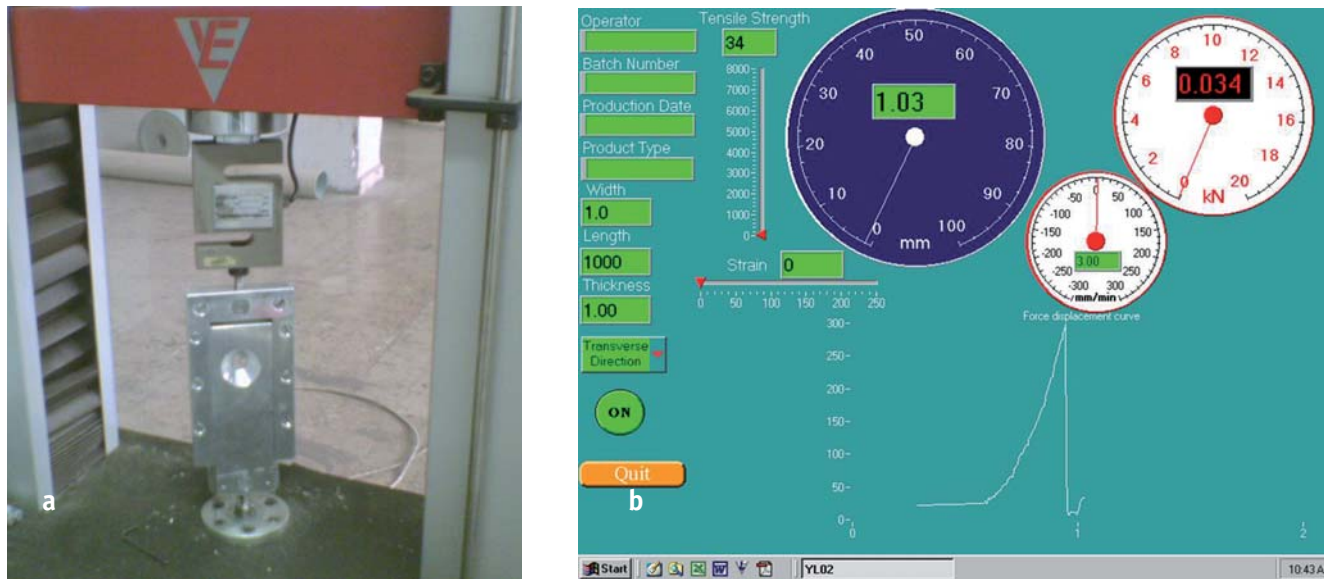
Figures 4a and 4b. Universal testing machine (a) and computer monitoring of the test values (b).
